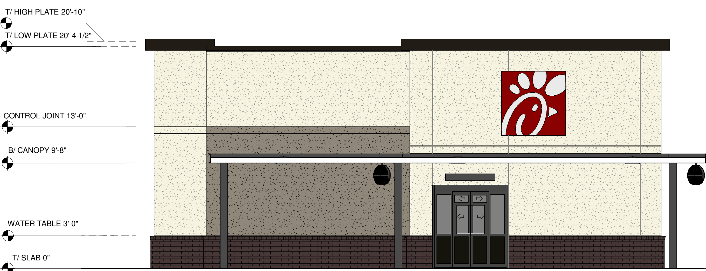
B2 NORTH EXTERIOR ELEVATION 3/16" = 1'-0"
