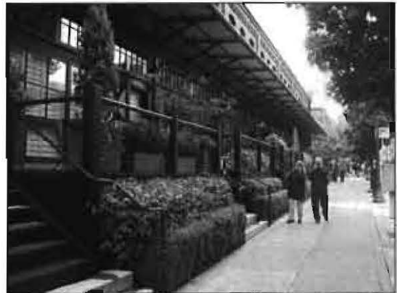
When residential development is located at street level, the ground flow should be elevated above street level or set back from the sidewalk with landscaping along the street frontage.
